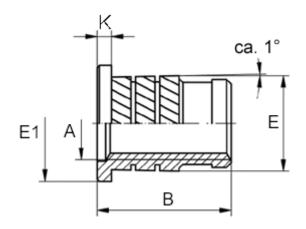
Female thread A = M2Flange diameter E1 = 4.8Flange heigth = 0.6Length B = 4.6Min distance to edge = 1.6 Outer diameter E = 3.35Recommended bore diameter = 3.1
